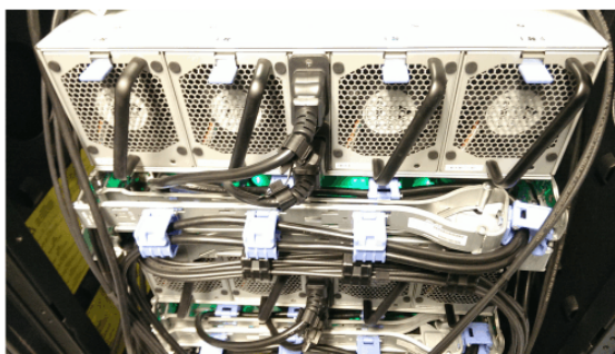
Figure 59. Power and SAS cable connections on the back of the enclosure
