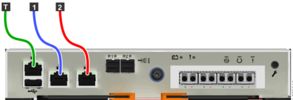
Figure 71. Connecting the Ethernet cables to a Storwize V5030E system
