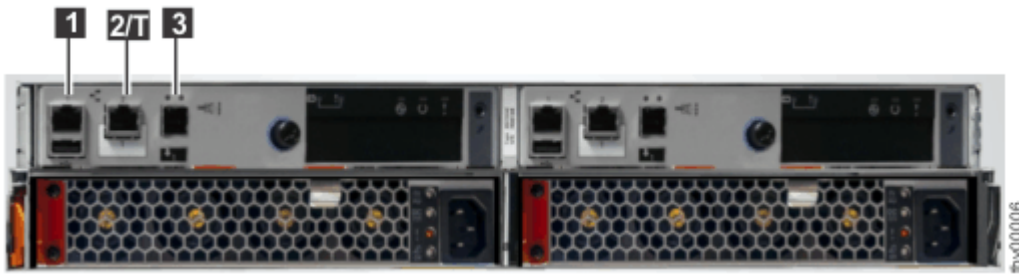
Figure 6. Data ports on the rear of the Storwize V5010E control enclosure
