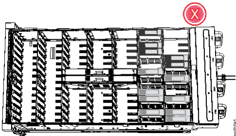
Figure 37. Incorrect drive installation
