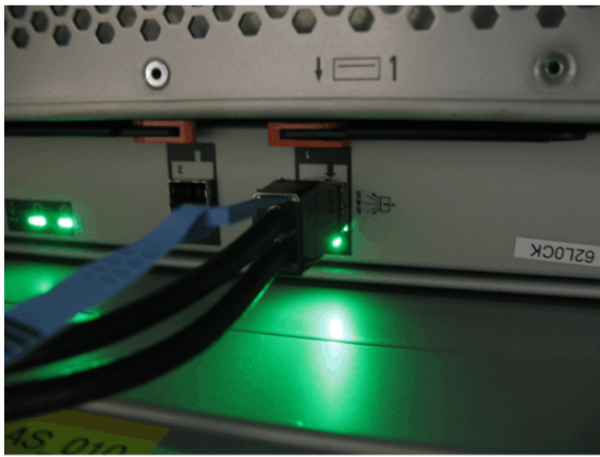
Figure 53. SAS cable correctly inserted into the SAS port
