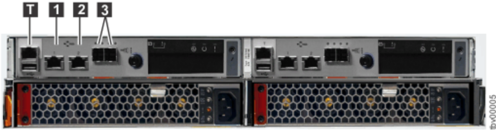
Figure 7. Data ports on the rear of the Storwize V5030E control enclosure
