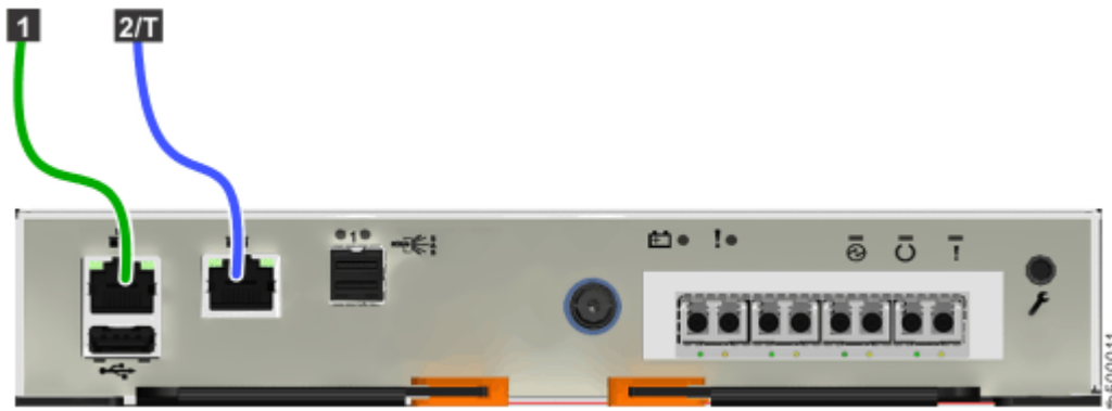
Figure 70. Connecting the Ethernet cables to a Storwize V5010E system
